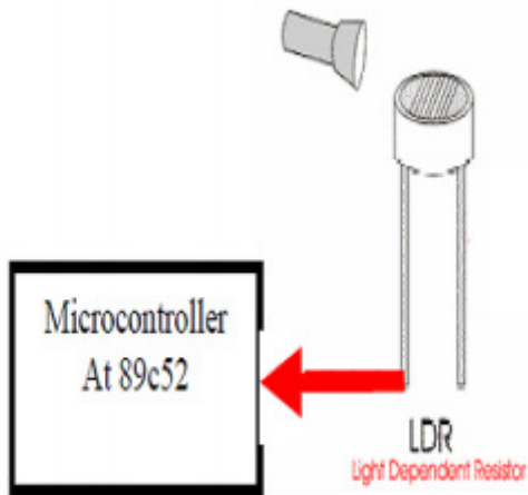
Figure6: Interface of LDR with Microcontroller
