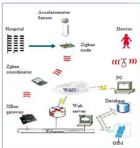
Figure 2.1: Patient health monitoring using Zigbee technology
