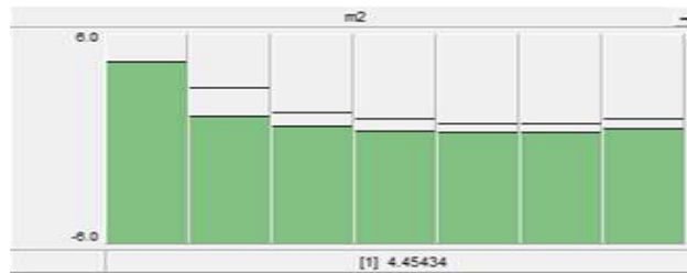
Fig 12: Harmonic content of voltage in phase B
