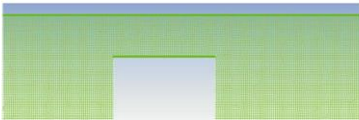
Figure 5: Computing grid for the gland labyrinth.
