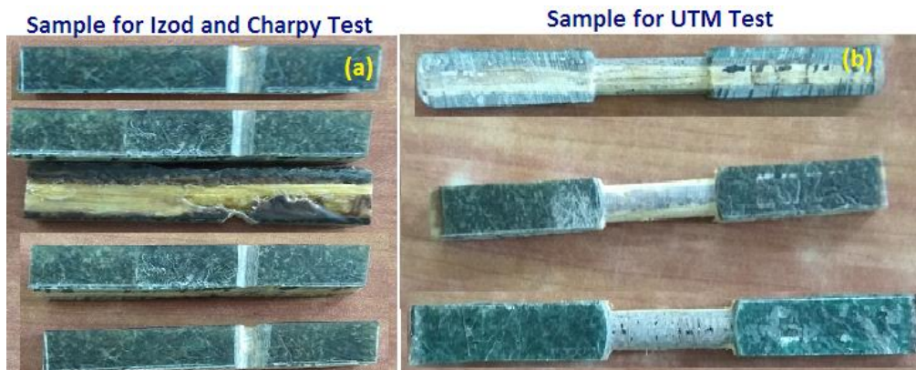
Fig. 3.4 (a) shows the sample of Izod and Charpy test and in (b) demonstrate the sample of UTM test.
