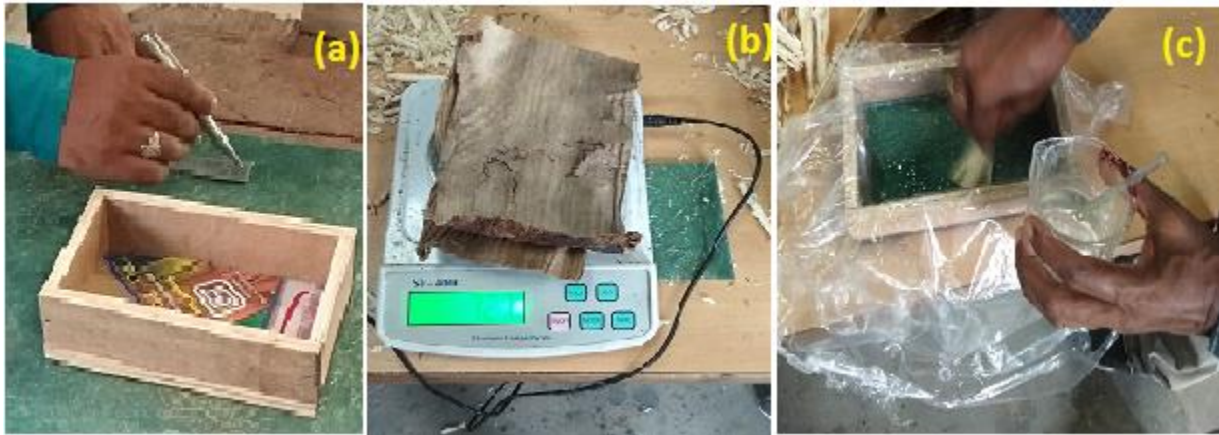
Fig.3 (a) preparation of wooden mould,(b) weighing machine for measuring different raw materials used in composites and in (c) initial set up for composites is shown.
