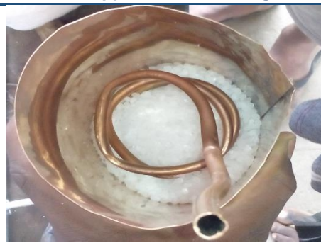
Fig.2: inside view of heat exchanger with paraffin
