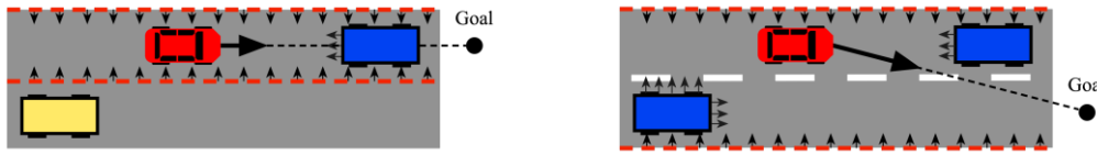
Fig. 7. Potential field generated by following driving intentions: (a) a case in which the driving intention is keeping, (b) a case in which the driving intention is changing and arrival, and (c) a case in which the driving intention is adjustment. The red vehicle represents the target, the blue one generates repulsive potential energy, and the yellow one does not generate repulsive potential energy. The red line denotes a sideline that generates repulsive potential energy.
