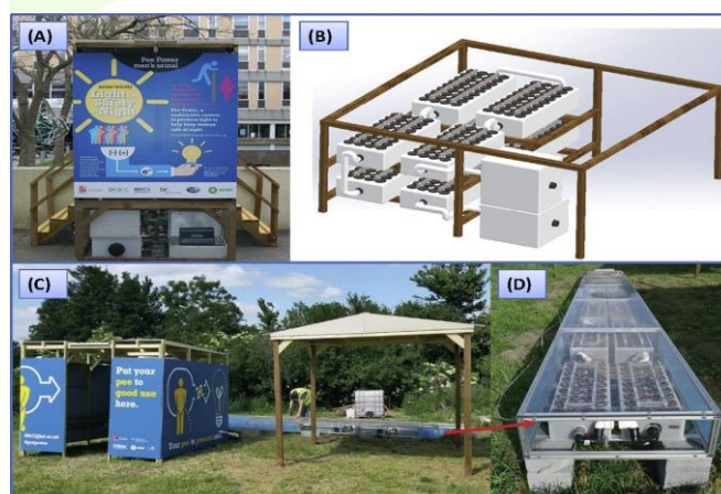
Fig. 5 Stacking the ceramic-based MFCs applied for indoor lighting; (A) 288-MFC stack trial in the UWE campus, (B) 3-D representation of 288-MFC stack with the inlet and outlet tanks underneath the urinal, (C) 432-MFC stack trial in Glastonbury Music Festival, (D) 432-MFC stack arranged in 12 modules [35].
