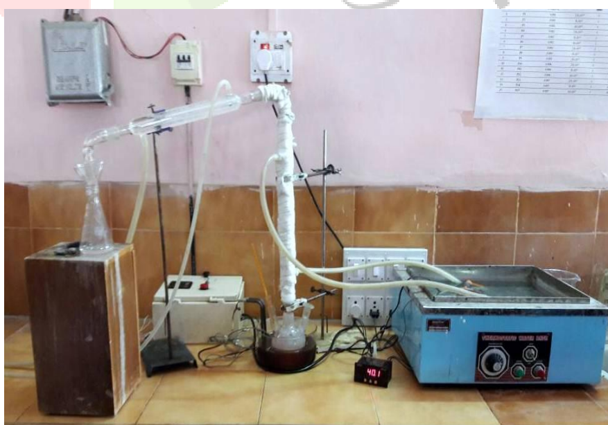
Figure.3: Fixed bed adsorber column
