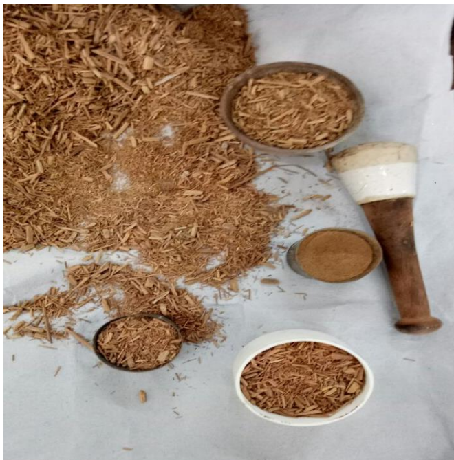
Figure 3: Dry bamboo samples placed in crucibles to carbonize in muffle furnace.
