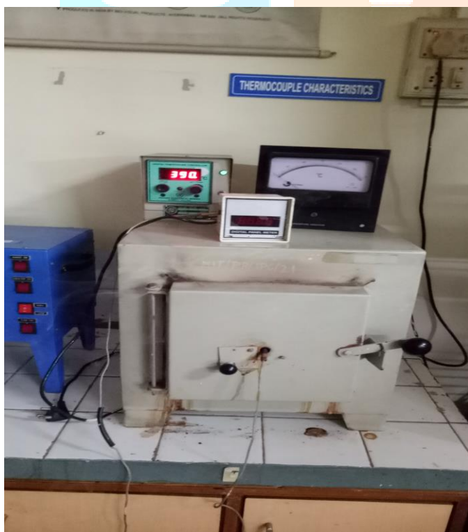
Figure 1: Dry bamboo samples subjected to muffle furnace at temperature of 380-400 C.
