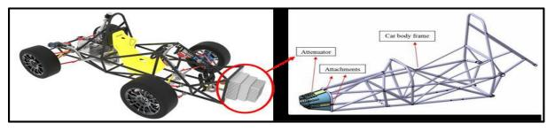
Fig. 1 Impact attenuator attachment to front bulkhead.
