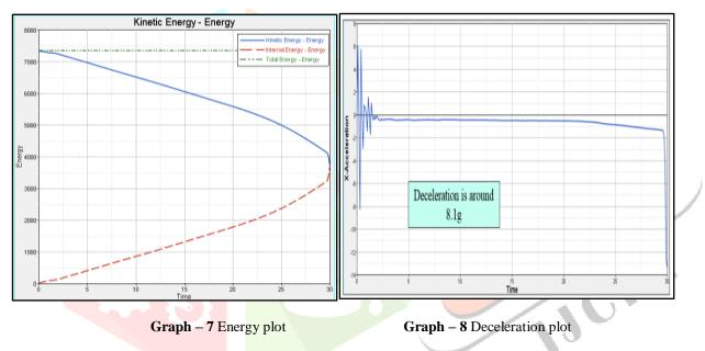
It is clearly visible from above plot that the peak deceleration is around 8.1g and it is 60% less than the FSAE requirement which is 20g. So this Honeycomb impact attenuator model with aluminum material (Case-IV) is meeting FSAE requirements.
