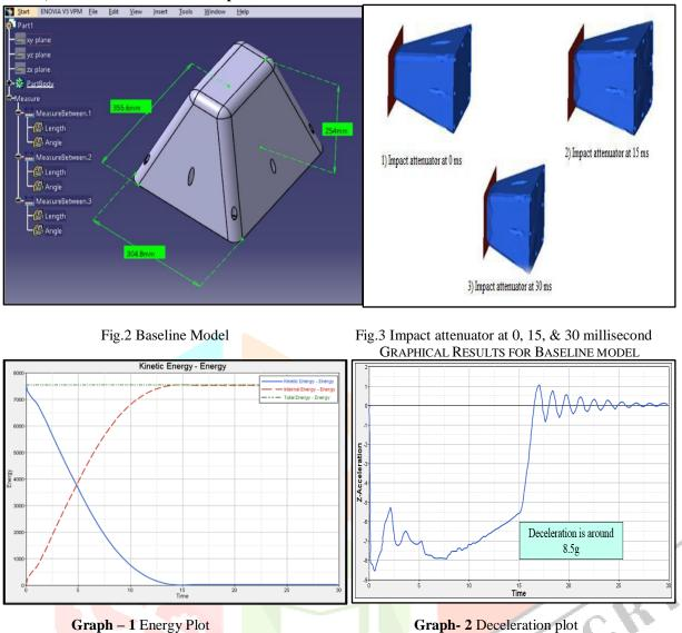
It is clearly visible from above plot that the peak deceleration is around 8.5g and it is 57.5% less than the FSAE requirement which is 20g. So this baseline impact attenuator model with aluminum material is meeting FSAE requirements.
