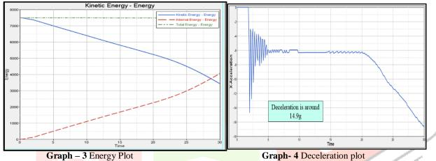
It is clearly visible from above plot that the peak deceleration is around 14.9g and it is 25% less than the FSAE requirement which is 20g. So this Honeycomb impact attenuator model with aluminum material (Case-II) is meeting FSAE requirements.
