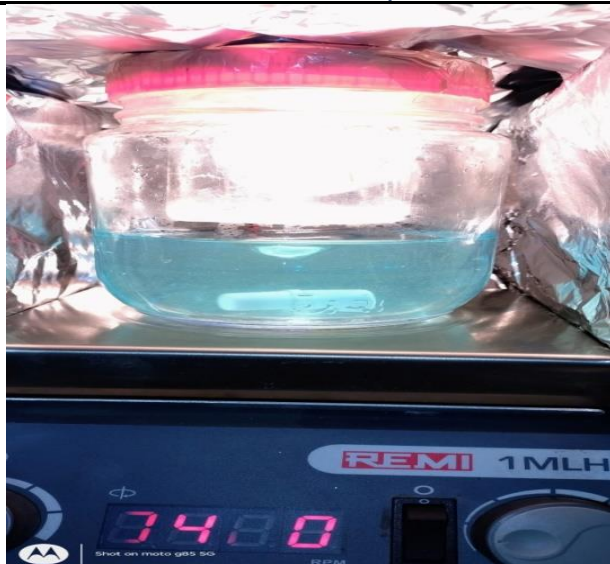
Fig. 6 Typical Photocatalytic Degradation using Methylene blue dye
