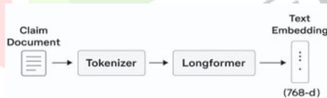
Fig. 1. Claim text embedding pipeline using Longformer
