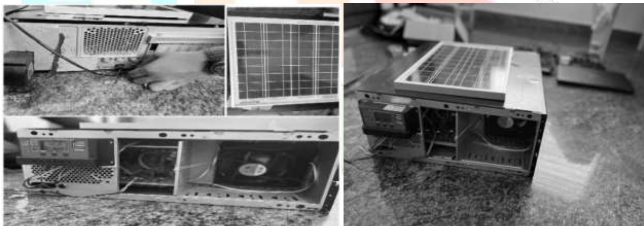
Figure 3: An implemented model of solar energy based air purifier with air quality monitor for vehicles
