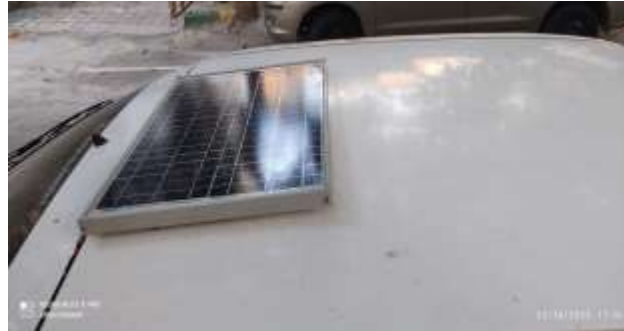
Figure 7: Placement of solar panel for solar energy based air purifier with air quality monitor for vehicles
