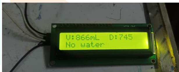
Figure 5. 1.1 Result of Fuel Analyzer with NO water present
