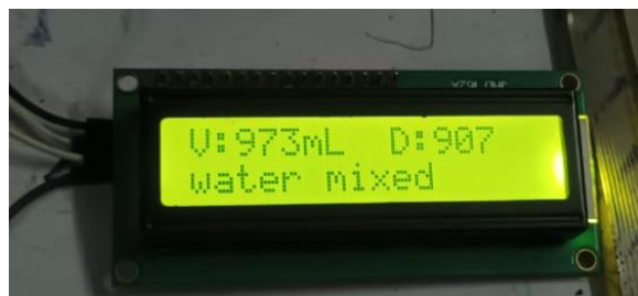
Figure 5.1.3 Result of Fuel Analyzer with water mixture present
