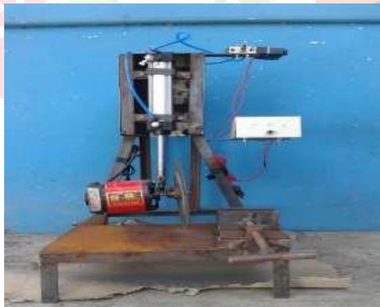
Fig.1 .The typical pipe cutting machine
