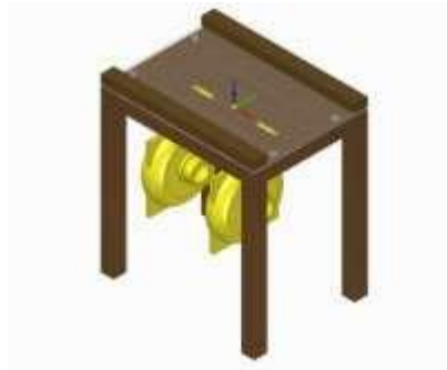
Fig: 2.1: Contactless Air Conveyor (Isometric View)
