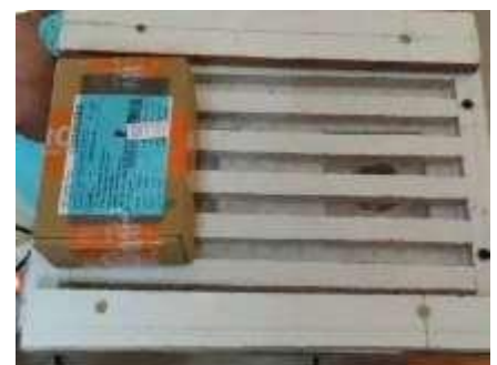
Fig: 2.5: Contactless Air Conveyor's Blower & with Conveying Product
