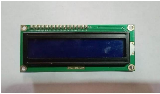
Figure-5: A 2 by 16 LCD display
