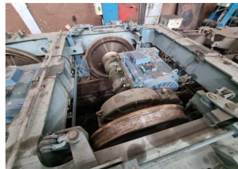
Fig. 2. Traction Motor arrangement in chassis (Diesel loco shed Ghorpadi Pune)
