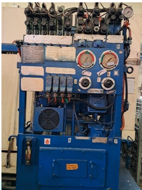
Fig2. Photograph of Hydraulic Clamping system employed in BFW SPM machine considered in the present study.
