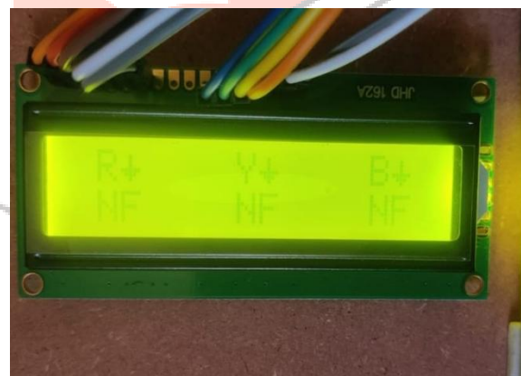
Fig.3: NF (Not Found) which means the cable is not having any fault
