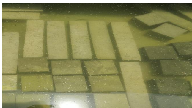
Figure 3.2: Curing of Rice Husk Ash Concrete cubes
