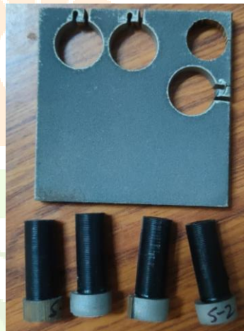
Figure 5: Samples used for wear testing
