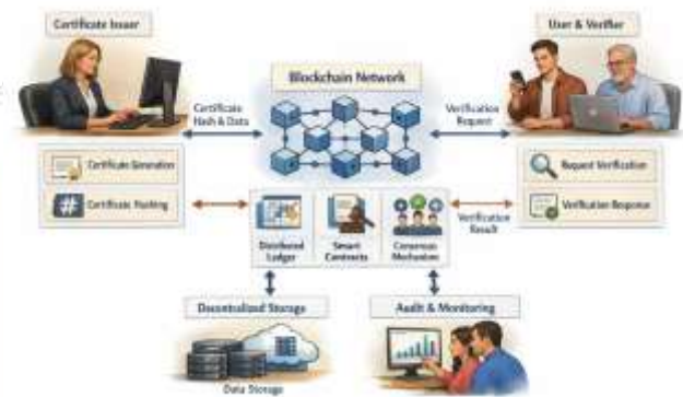
Fig. 1. General Architecture of Blockchain-Based Certificate Authentication Systems
