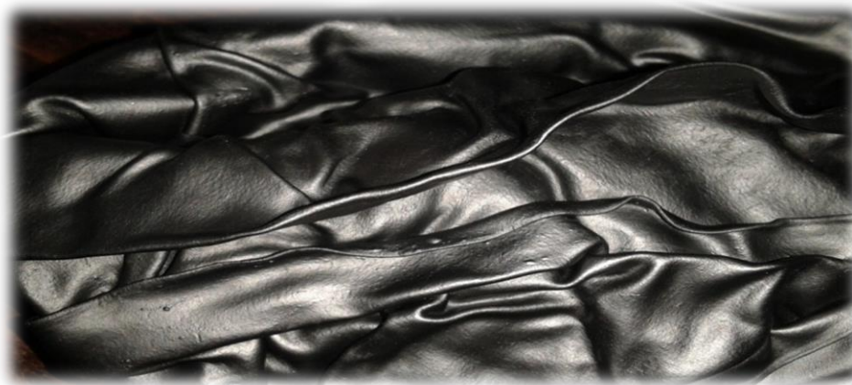
Figure 5. Blended sheet of nanocomposite material with Nano Graphene Platelets
