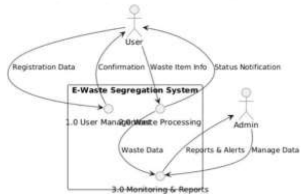
Fig. 4. Data flow diagram of the proposed WasteWise system
