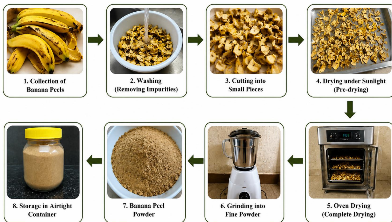
Fig. 1. Preparation Process of Banana Peel Powder for Wastewater Treatment
