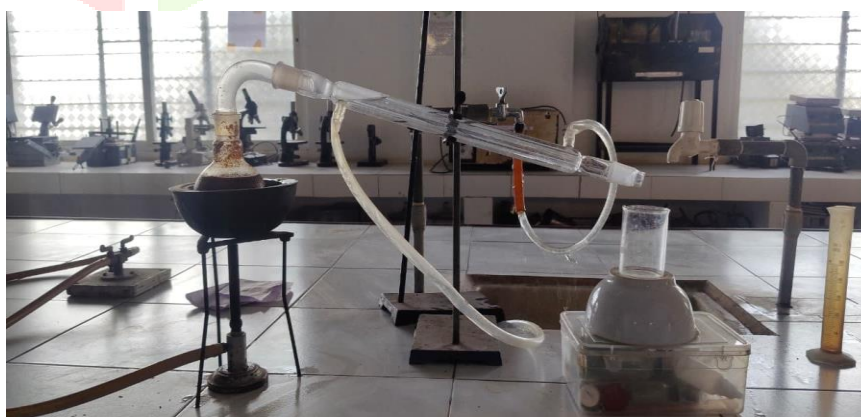
Fig no 5 (Clove extract Obtained By Hydro distillation process)
