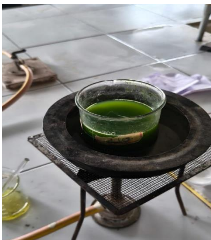
Fig no 6 (Neem Extract Evaporation to remove water)
