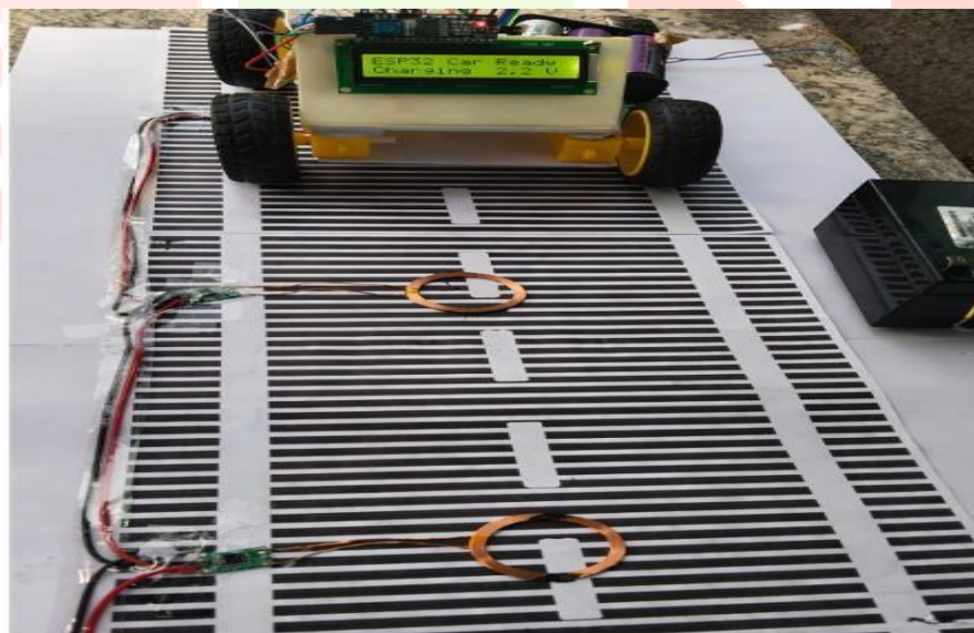
Fig 4.2 Successfully charging the battery of EV's through the coil
