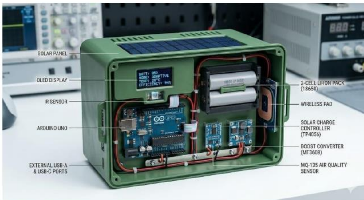
Fig 1 : Power bank prototype internal structure
