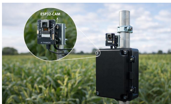
Fig. 8: Physical hardware setup — ESP32-CAM and field enclosure.
