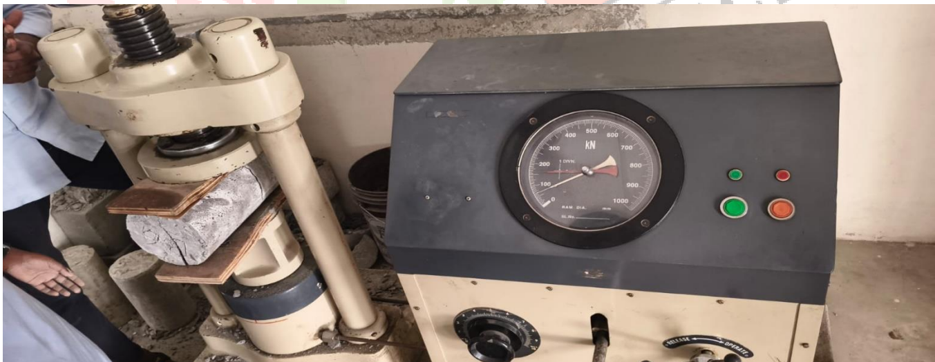
FIGURE NO:5 Concrete Specimen Placed In a Compression Testing Machine To Measure Compressive Strength
