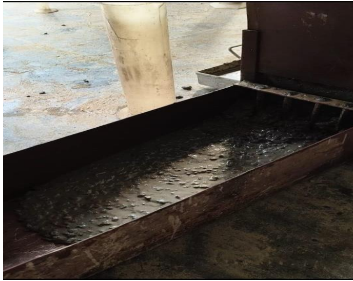
FIGURE NO:2 Flowability test of SCC concrete through Reinforcement bars using L-Box Setup
