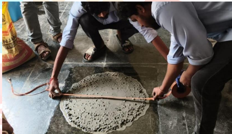
FIGURE NO :1 Measuring Flowability of SCC
