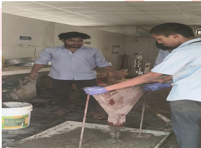
FIGURE NO: 3 Measuring time duration for flowability of SCC using V-funnel
