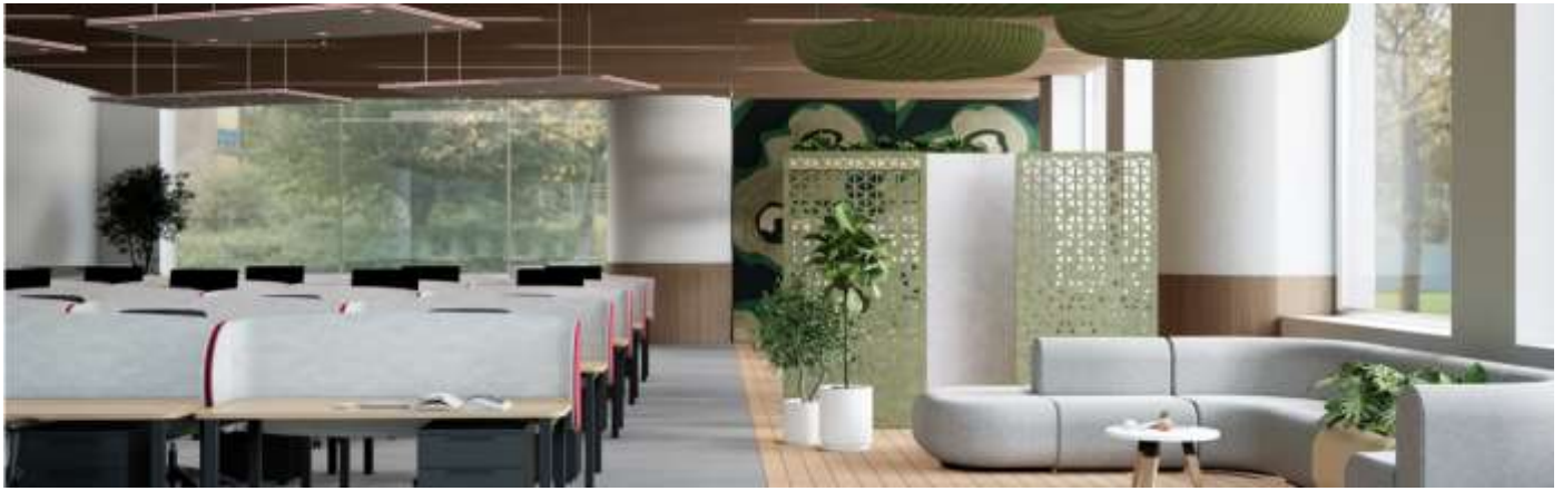
Figure 6: Example of a modern open-plan office using various acoustic strategies, including suspended round panels for controlling reverberation, ceiling baffles that absorb sound, fabric-covered partitions to maintain speech privacy, and strategic spatial zoning to reduce noise distractions. [36]
