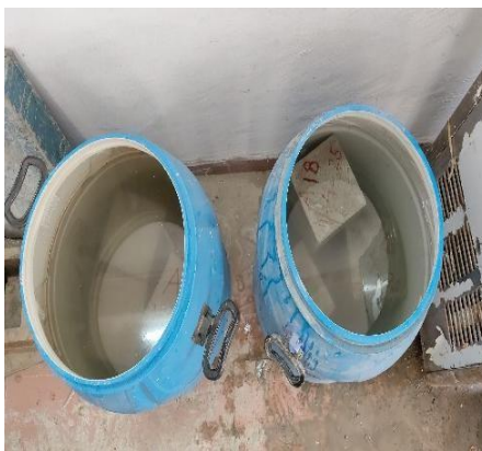
Fig 4/5/6: Curing in Water/Sodium Chloride/Sulfuric Acid
