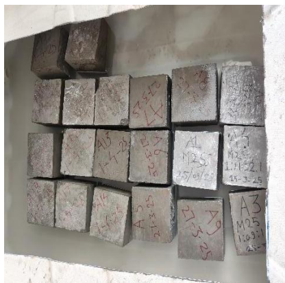
Fig 4/5/6: Curing in Water/Sodium Chloride/Sulfuric Acid
