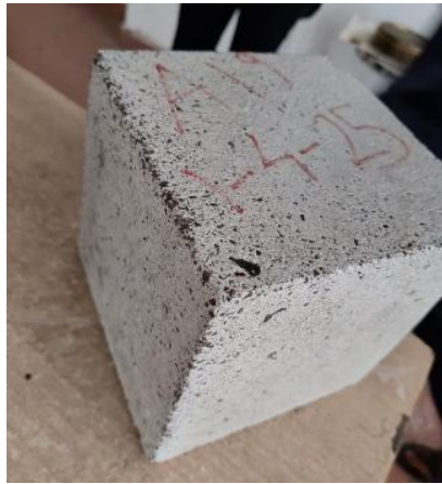
Fig 1: After 28 days curing in sulfuric acid (2.5 % Concentration) concrete cube surface started to rough and porous
