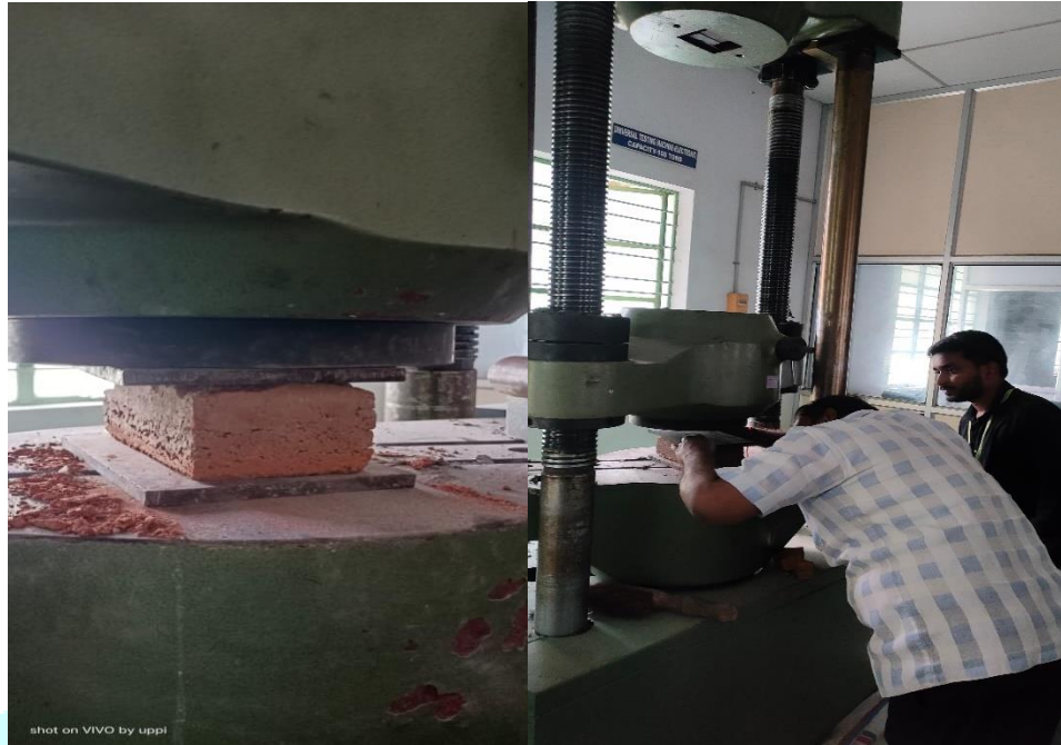
Figure 6 Set up of compressive strength testing of brick
