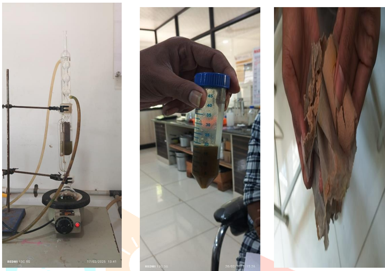
Fig.3.2. Soxhlet extraction setup and Ethonolic extract collection
