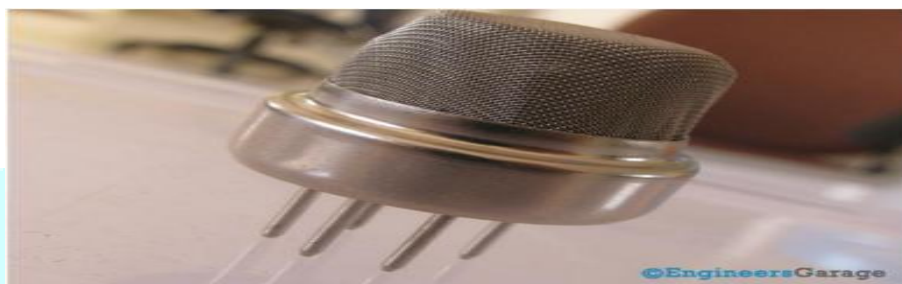
Fig 1: Gas sensor for alcohol detection
