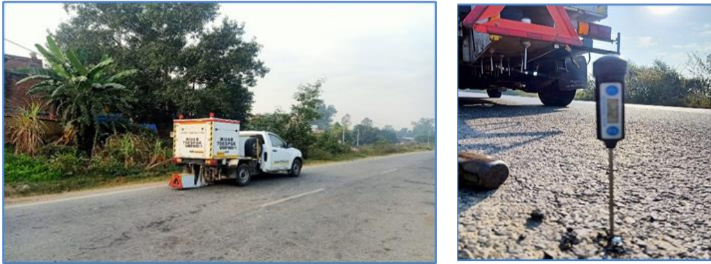
Figure 3: Deflection and Temperature measurements
