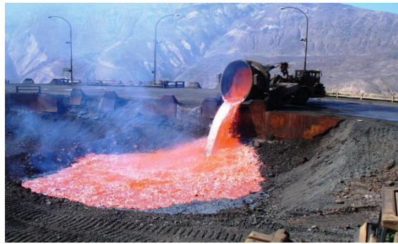
Fig.1. Removal of steel slag while steel manufacturing
