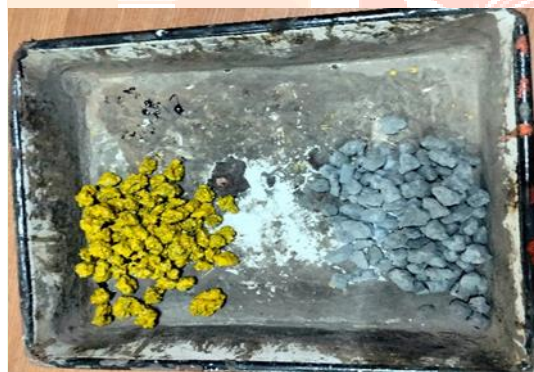
Fig.9. coating of oil paint and cement paste on the steel slag
