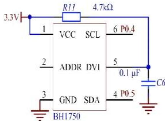
BH1750 is available as a 5-pin IC. Pin description of the IC is given below-
