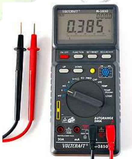
A millimeter or a multimeter, also known as a VOM (Volt-Ohm meter), is an electronic measuring instrument that combines several measurement functions in one unit. A typical millimeter would include basic features such as the ability to measure voltage, current, and resistance. Analog millimeters use a micro
