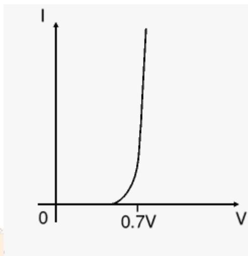
The Peak Reverse Voltage (PIV) of silicon types is available up to 1000 volts or more. They can also carry up to 100A DC current. In typical applications, it is advisable to ensure that it operates within the maximum ratings specified by the manufacturer and apply the Failure Mode and Effects Analysis to the device. The temperature of the device is one of the more important parameter to consider. Heat sinks may be used where they have to handle large amount of power.
