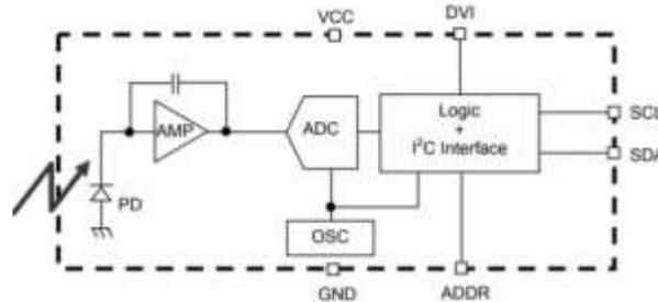
Ambient light sensors contain a photodiode that can sense light and convert it into electricity. Light is measured depending upon its intensity. From the block diagram, PD is the photodiode which is used to sense the light. Its response is approximate to the human eye response.
