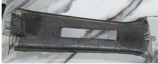
Fig. 5.3 Carbon fiber reinforced B-Pillar trim
