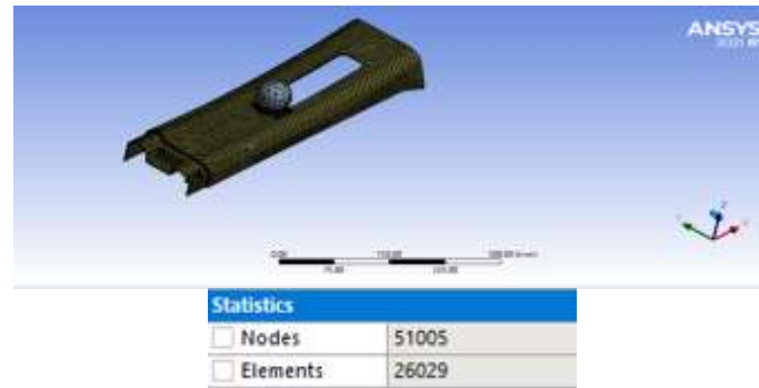
Fig. Meshing Details of E glass fiber composite B-Pillar Trim
