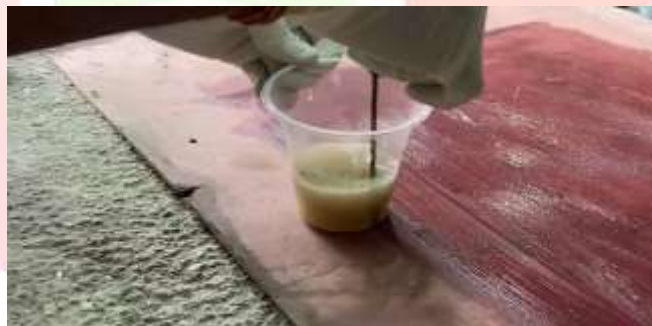
Fig. 5.1 Preparation of Resin and hardener
