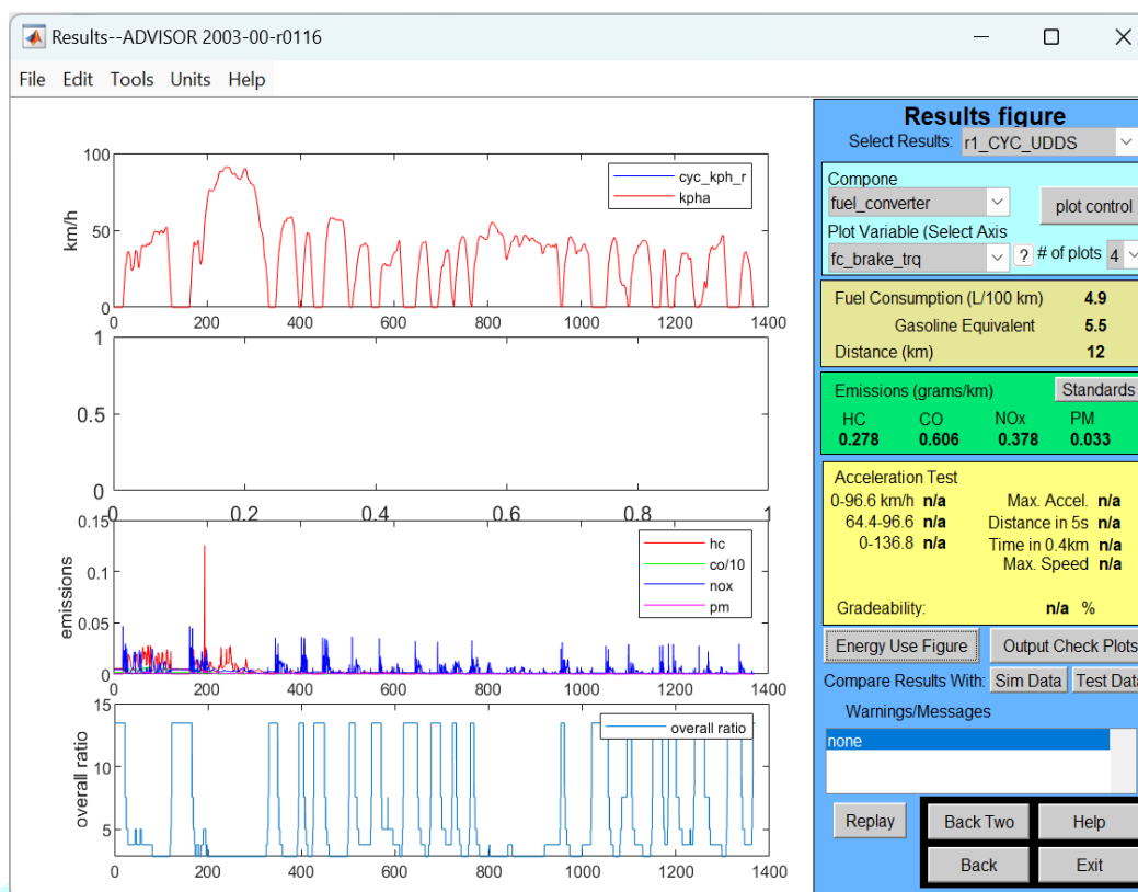
Figure 7: ADVISOR result for ICEV on UDDS cycle at 10 °C
