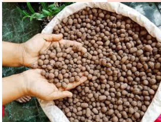
Fig 2 : Lightweight Expanded Clay Aggregate (LECA) Balls
