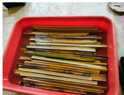
Figure 3: Bamboo strips soaked in NaOH solution for alkali treatment
