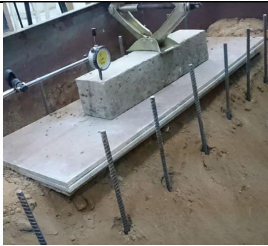
(c) Micro pile embedded in soil
