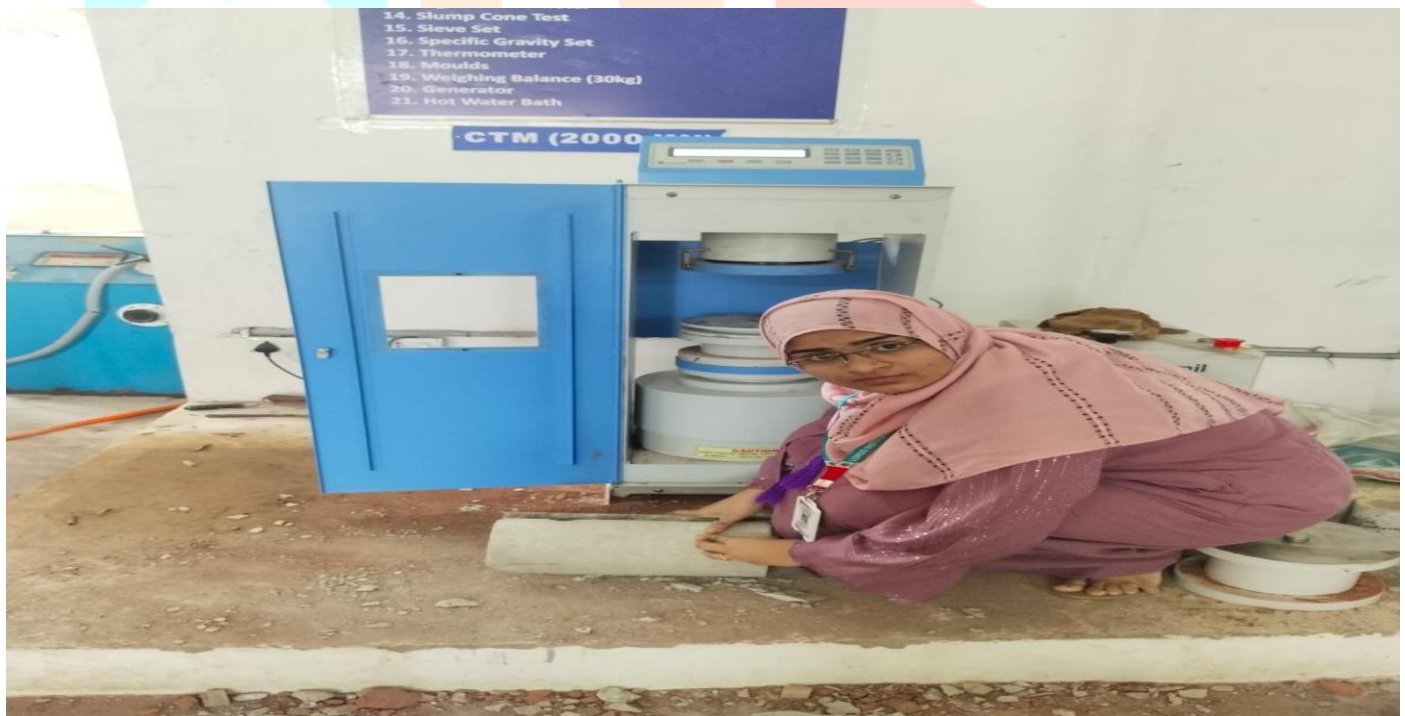
FIG: 6.2 Split Tensile Strength Test
