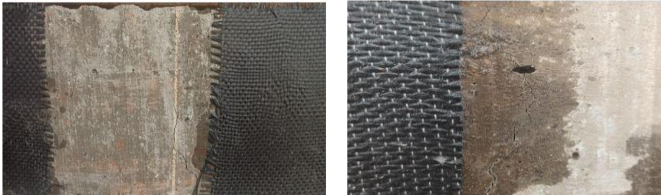
Figure: 6.3.4 Flexural strength of M25 Beam Wrapped with CFRP at 50 mm Interval (Average strength of 3 prisms)
