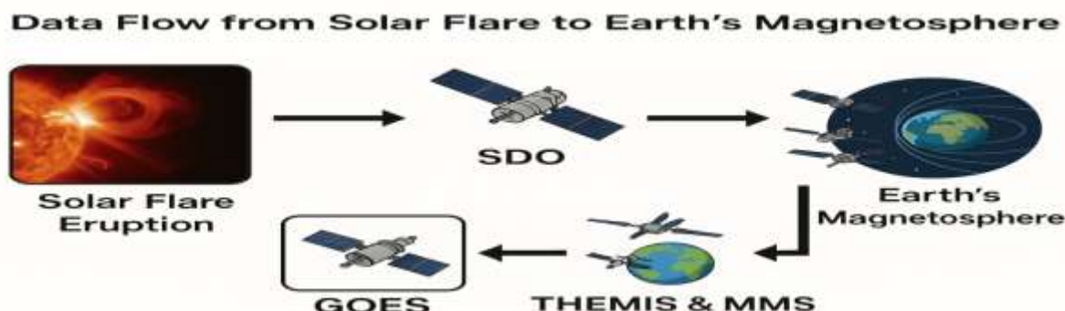
figure 3: data flow from a solar flare eruption to earth's magnetosphere, showing real-time monitoring by SDO, GOES, and THEMIS & MMS satellites to build a complete event timeline
