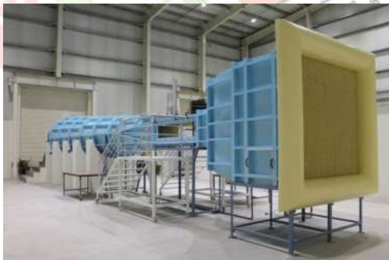
Figure 7 Subsonic wind tunnel Velocity up to 80 m/s
