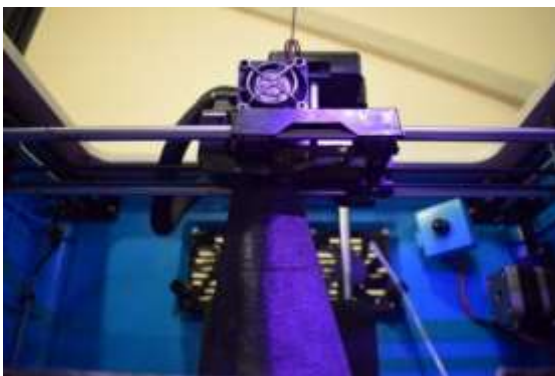
Figure 5 Fused Deposition 3D printing setup
