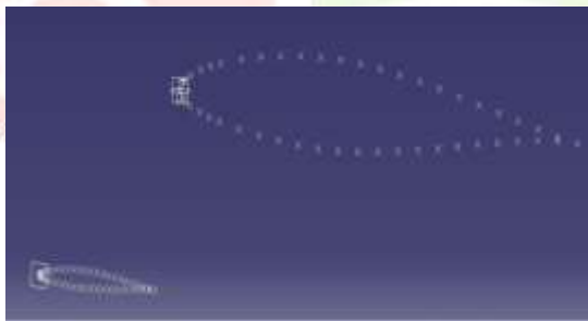
Figure 2 Generation of Coordinates at root and tip with predefined macros in CATIA V5.
