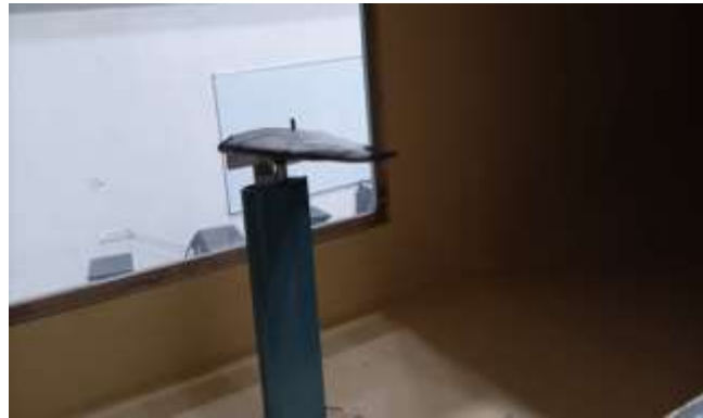
Figure 9 Wing is placed on the wind tunnel
