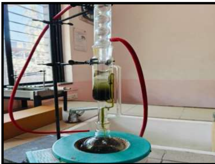
Fig no.1: Extraction of moringa leaves using Soxhlet assembly
