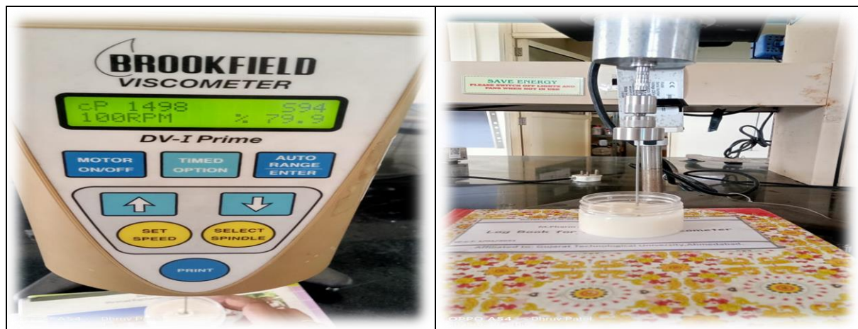
Figure 11 – Viscosity testing by Brookfield Viscometer
